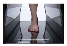
Each of the four lasers projects a line onto the foot from several angles. The eight monochrome cameras capture the laser projections.
